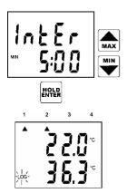
Now instrument displays adjusted storing interval. To modify the storing interval use arrow keys. Interval 10 sec is displayed as **MIN 0:10**, minute intervals are displayed as **MIN x:00** and hour intervals as **x:Ho**. Confirm adjusted interval by pressing ENTER key. Notice: if manual logging mode is selected, this menu item is skipped (there is no interval adjustment).
