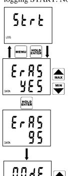
If it is needed to clear the memory before logging start, first it is necessary to select menu item logging START (symbol Strt) and confirm by pressing ENTER key.
