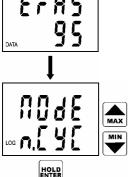
Clearing procedure is in progress. It takes approximately 16 s and the duration is indicated by displaying of already cleared memory in % (digits 0 to 100).
