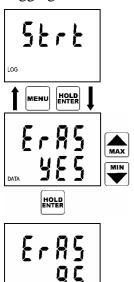
If it is needed to clear the memory before logging start, first it is necessary to select menu item logging START (symbol Strt) and confirm by pressing ENTER key.
