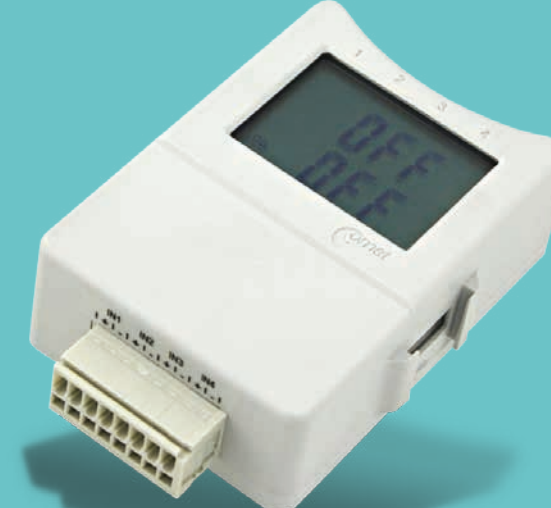
Datalogger S7021 reads and records data from electrometer.
