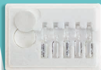
HM023 - set of 5 humidity standards 10% RH with 5 application pads.
