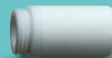
F5300 - teflon sensor cover with increased resistance against splashing water. Cover is not suitable for applications with risk of condensation. Filtering ability 0.025mm.
